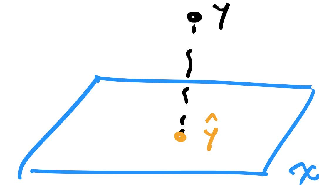
For a subspace  $\mathcal{X} \subseteq \mathbb{R}^n$ , the **projection** of a vector  $y \in \mathbb{R}^n$  onto the set  $\mathcal{X}$  is the closest vector  $\hat{y}$  in  $\mathcal{X}$  to  $y$ , in a Euclidean distance sense:
